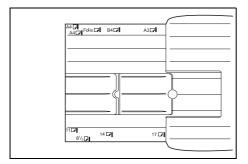
The paper sizes are marked on the ejected paper guide extension. Open ejected paper guides 1 and 2 as necessary to accommodate the size of the paper.
